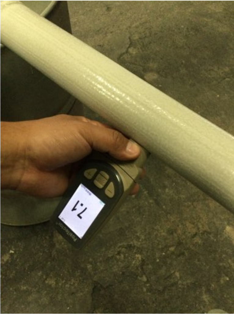
Photo Description: Epoxy dry film thickness measurement
