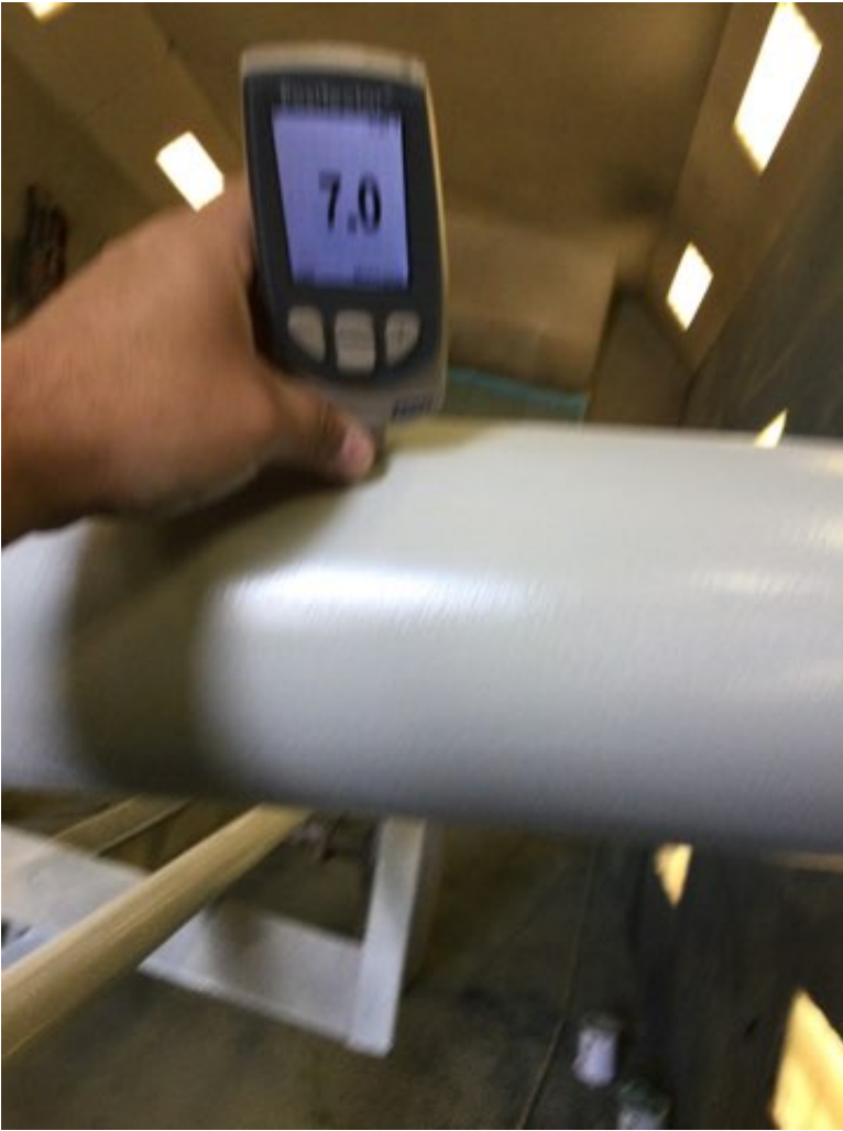
Photo Description: Epoxy dry film thickness measurement
