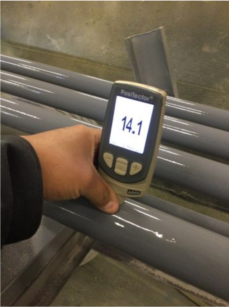
Photo Description: Polyurethane dry film thickness measurement
