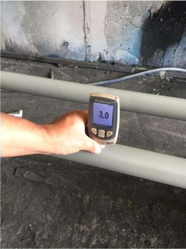
Photo Description: Zinc coating dry film measurement
