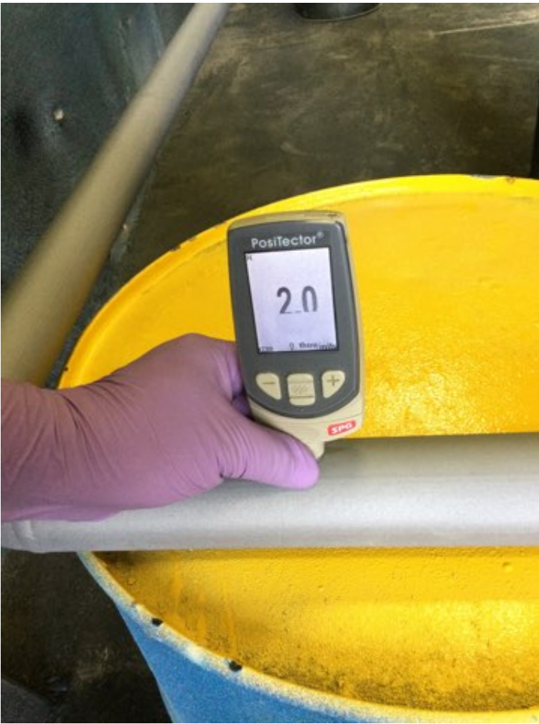
Photo Description: Grit blasted Surface profile measurement
