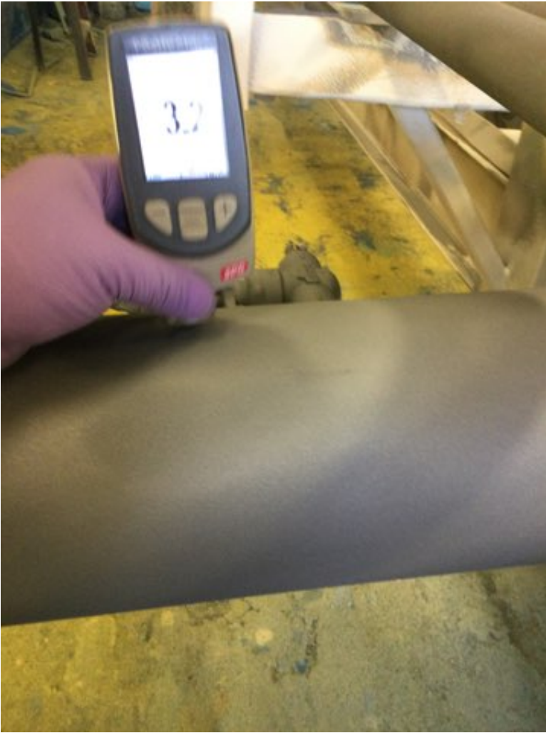
Photo Description: Grit blasted Surface profile measurement
