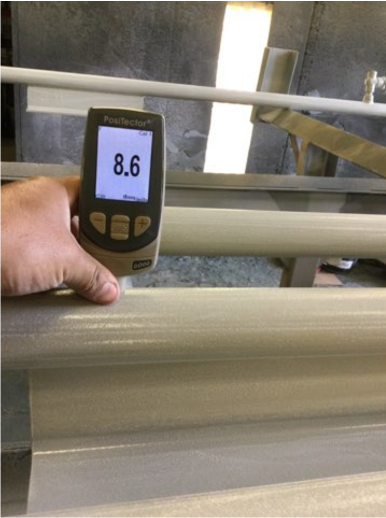
Photo Description: Epoxy dry film thickness measurement
