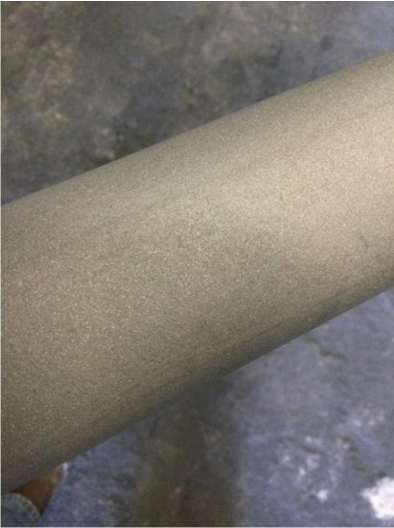
Photo Description: Grit blast closeup
