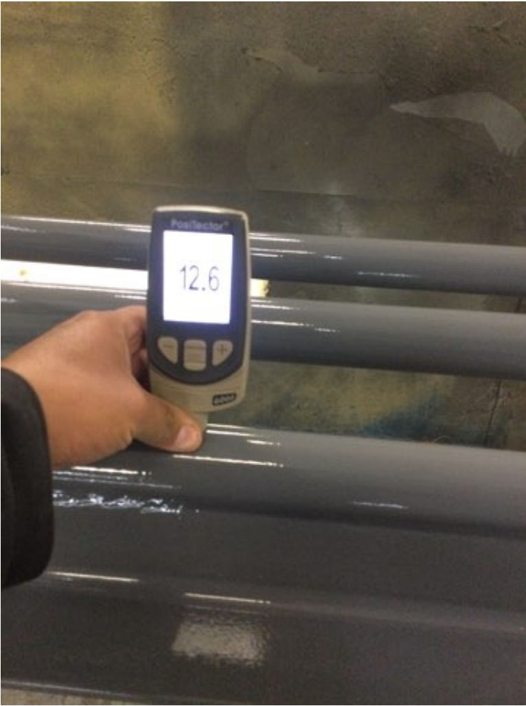
Photo Description: Polyurethane dry film thickness measurement
