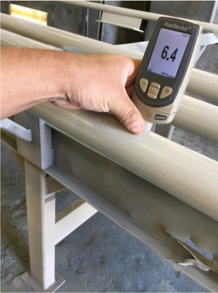
Photo Description: Epoxy dry film thickness measurement
