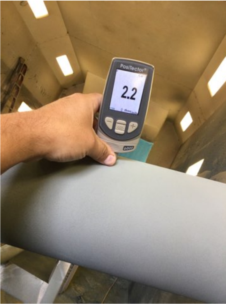
Photo Description: Zinc coating dry film measurement
