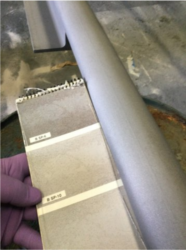
Photo Description: Grit blasted Surface visual comparison to SSPC -VIS 1 guide SP10 cleaning
