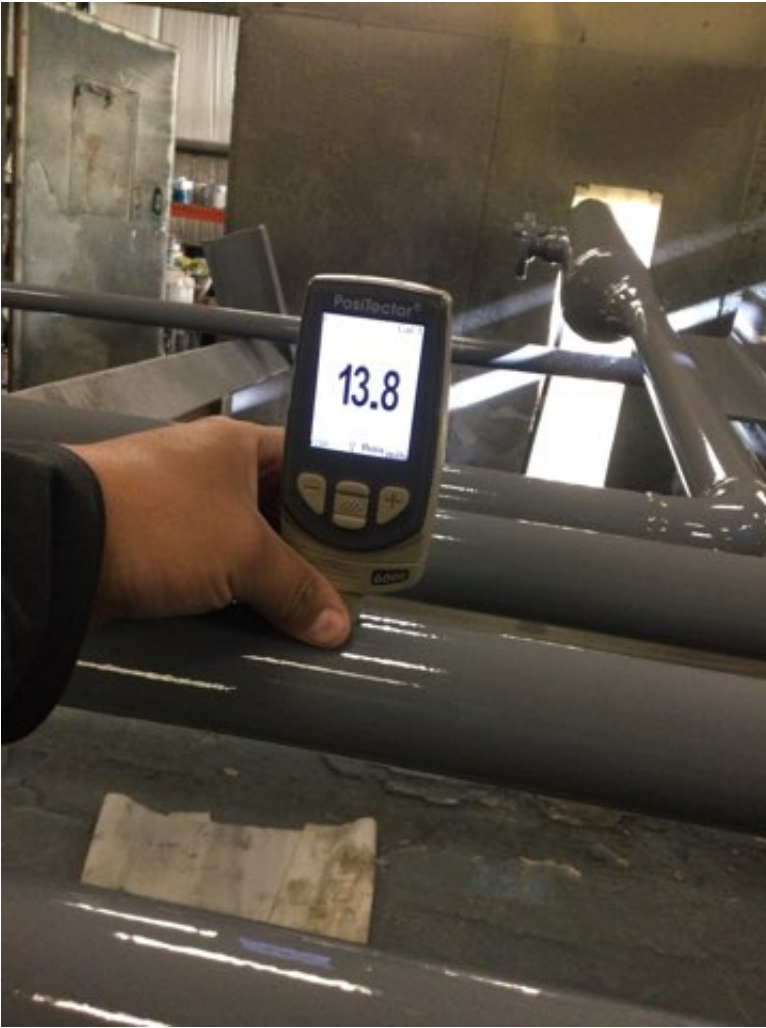
Photo Description: Polyurethane dry film thickness measurement
