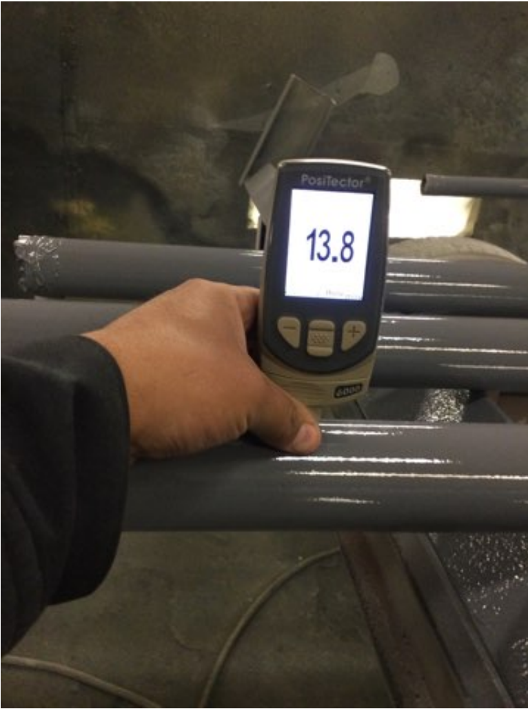
Photo Description: Polyurethane dry film thickness measurement
