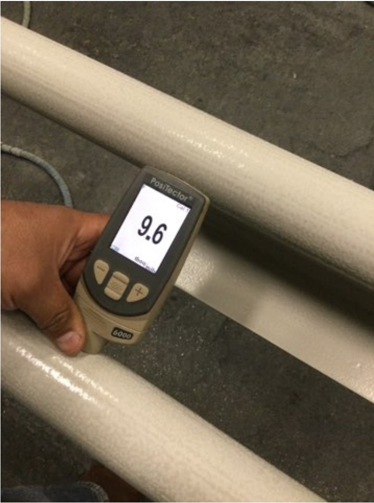
Photo Description: Epoxy dry film thickness measurement
