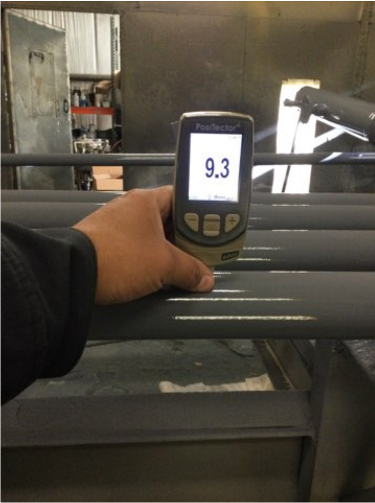
Photo Description: Polyurethane dry film thickness measurement
