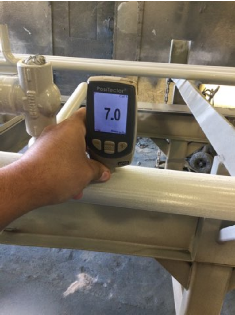
Photo Description: Epoxy dry film thickness measurement
