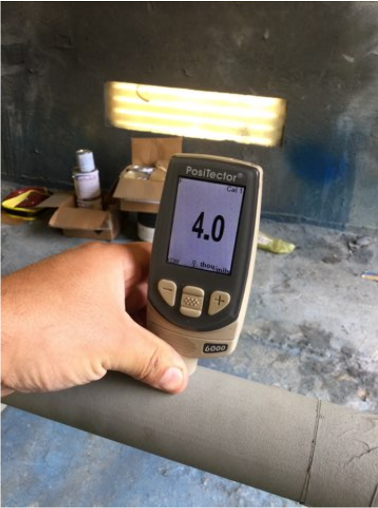
Photo Description: Zinc coating dry film measurement
