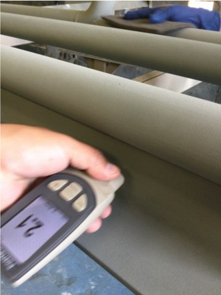
Photo Description: Zinc coating dry film measurement
