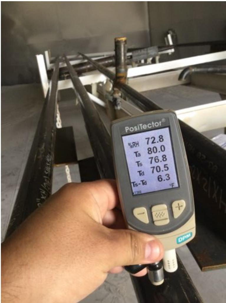
Photo Description: Immediately before grit blasting
