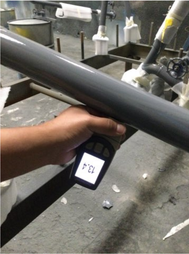
Photo Description: Polyurethane dry film thickness measurement
