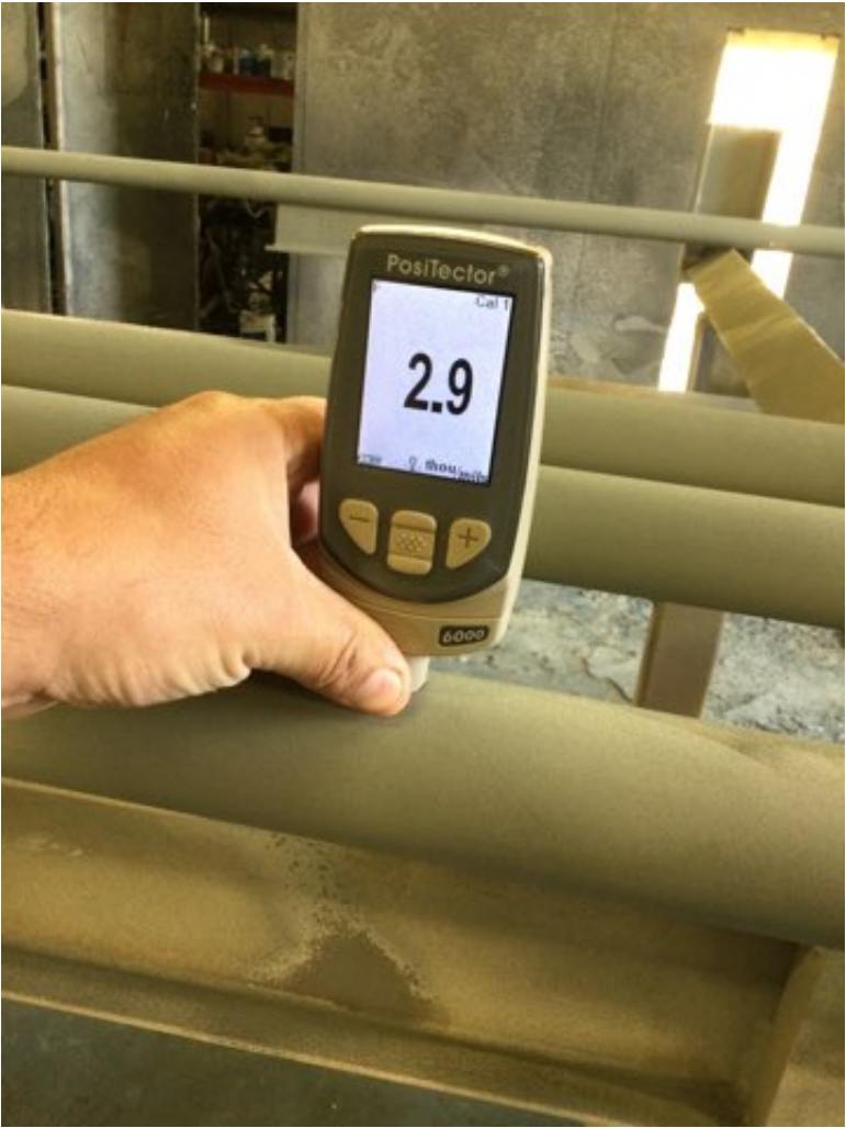
Photo Description: Zinc coating dry film measurement
