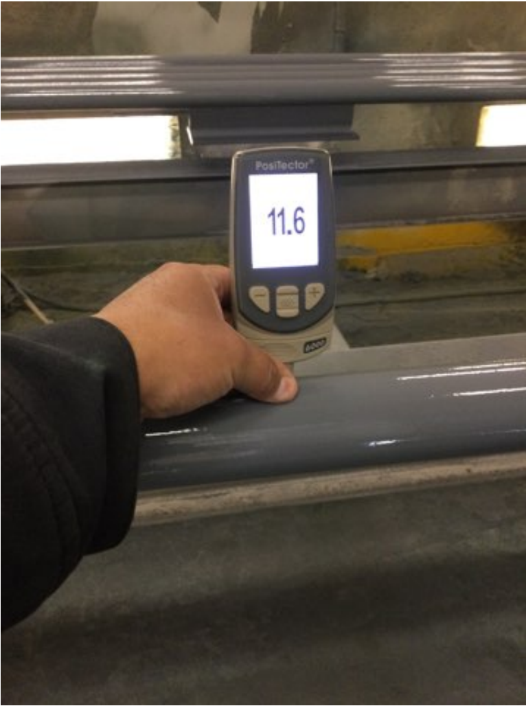
Photo Description: Polyurethane dry film thickness measurement
