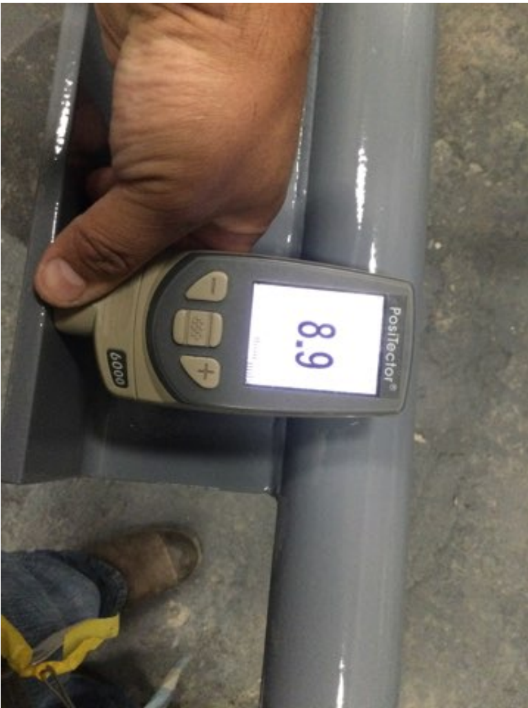
Photo Description: Polyurethane dry film thickness measurement
