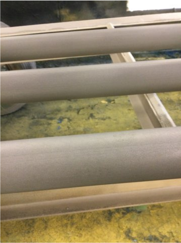
Photo Description: Grit blasted
