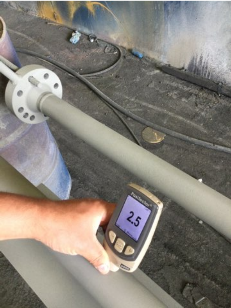
Photo Description: Zinc coating dry film measurement
