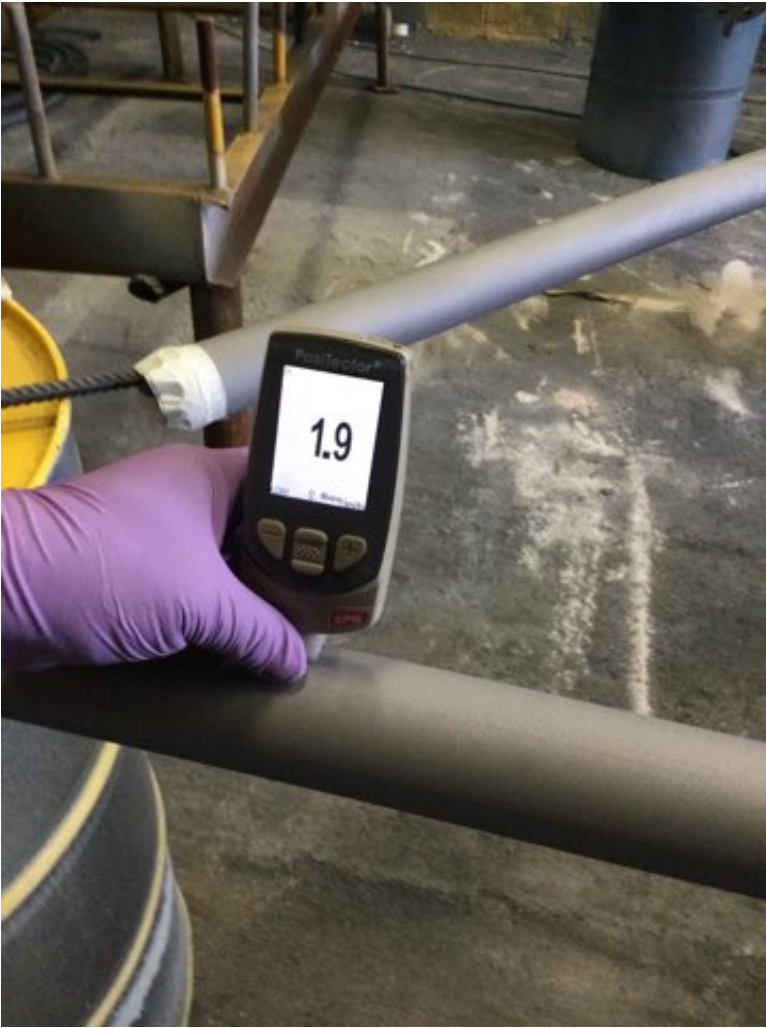
Photo Description: Grit blasted Surface profile measurement
