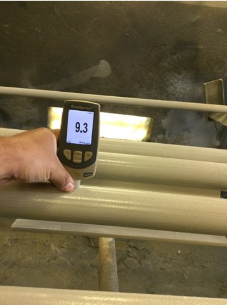
Photo Description: Epoxy dry film thickness measurement
