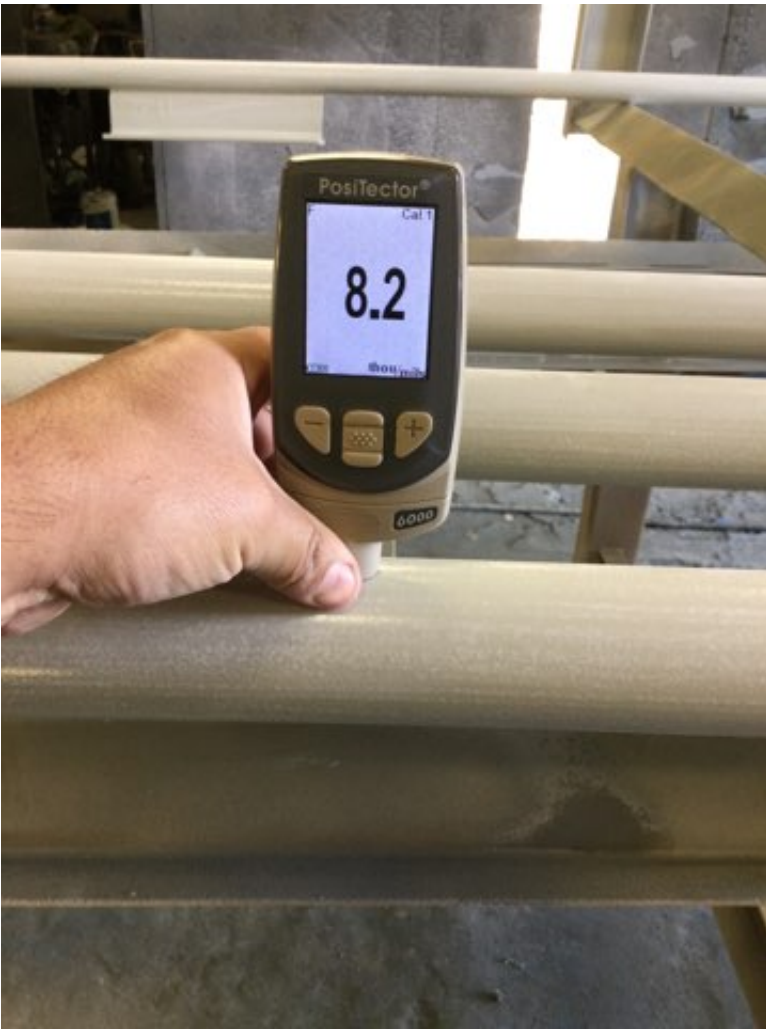
Photo Description: Epoxy dry film thickness measurement
