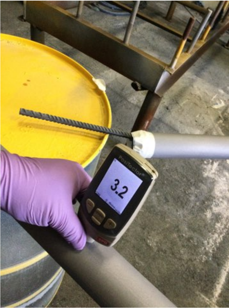
Photo Description: Grit blasted Surface profile measurement
